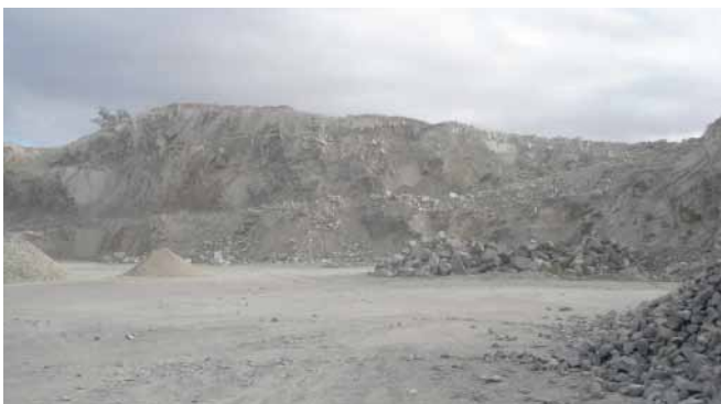
Figure 3: Capturing and stockpiling armourstone within a quarry
