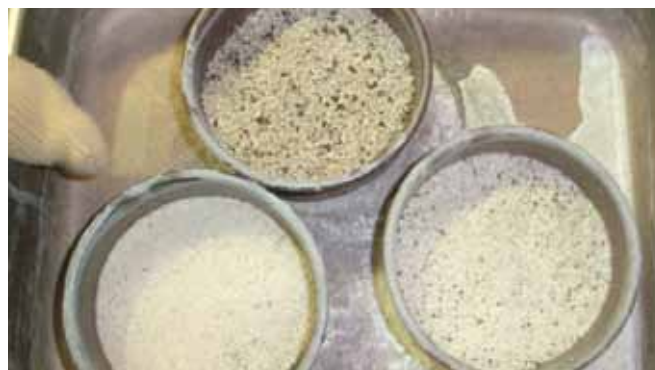
Figure 8: Sodium sulfate soundness bath and test portions after soaking
