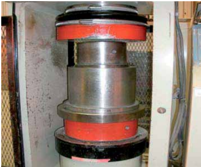
Figure 9: A Wet/Dry sample under test in a compression machine
